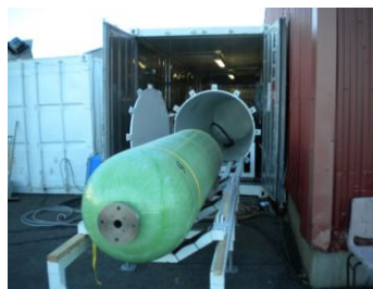
Fig. 5: CAPV undergoing fatigue testing
