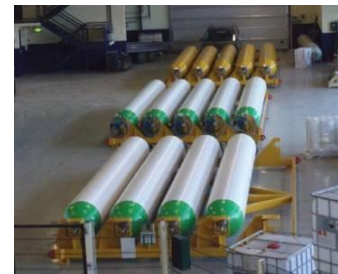
Fig. 2: Composite Air Pressure Vessel (CAPV).
